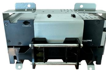
2. Take the 14-way connector on the vehicle interface harness and plug this into the relevant connection on the side of the interface.
